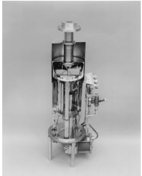
Fig. 4. X-band TWM internal cryogenic structure (courtesy of the Jet Propulsion Laboratory, California Institute of Technology).
